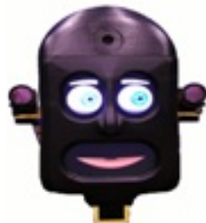
Fig. 1. BERT2’s expressive head. An embedded LCD screen generates gestures. Animated eyes communicate the direction of attention. The stereo vision system faceLAB from Seeing Machines TM is mounted on the side of the head for head and gaze tracking. A webcam is mounted centrally in the forehead for a wide angle view of the scene.
