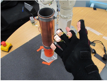
Fig. 6. Alternative setup for detecting when the user touches the cup.
